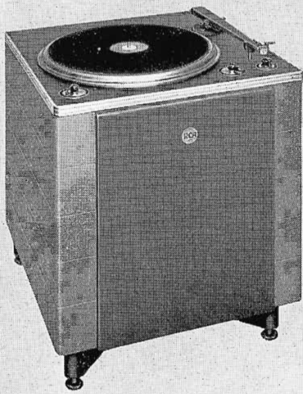
NEW BQ-2A 3-SPEED TURNTABLE designed specifically for 33½, 45 and 78 RPM operation. Low in price, but retaining highest performance characteristics. Simple, sure-fire drive mechanism with self-compensating rim drive. Smooth half-turn starting at any speed for easy cueing.
