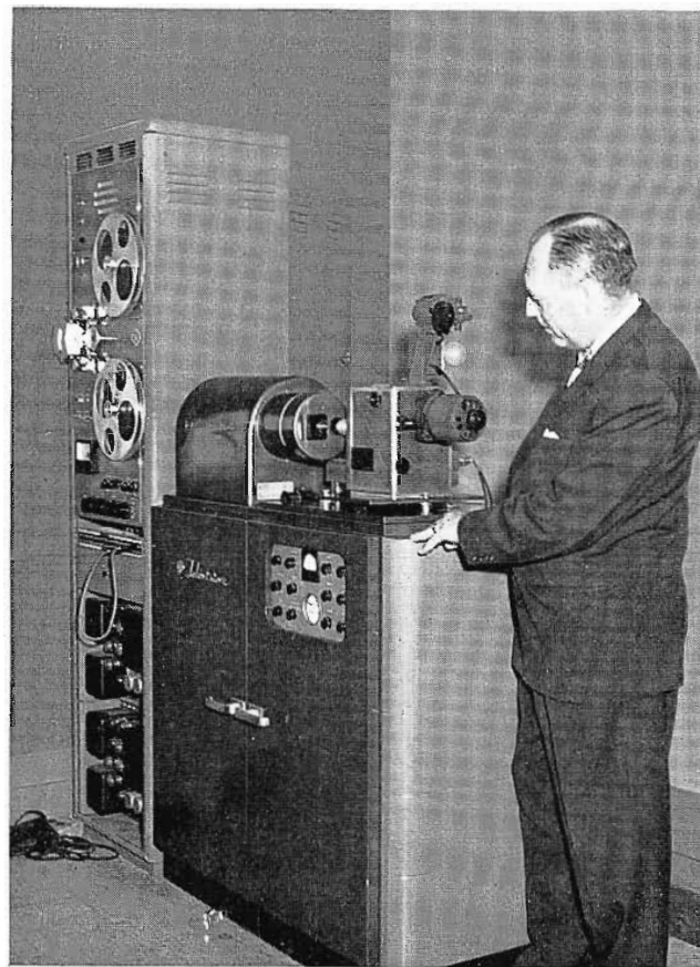
RCA TMP-20B kinephoto recording equipment. Kinescope films of WQED's most successful programs are produced here for national distribution through the Ford Foundation film center.
